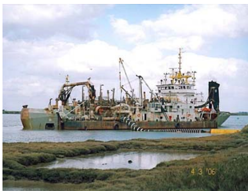
Photograph 8: The dredger pumps ashore the pollutant free mud from Harwich
